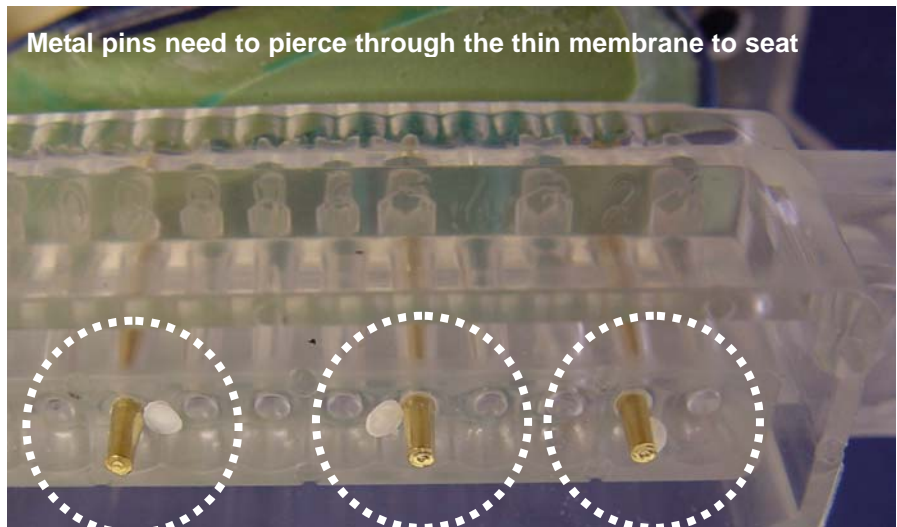
Use impression handle for pin insertion
