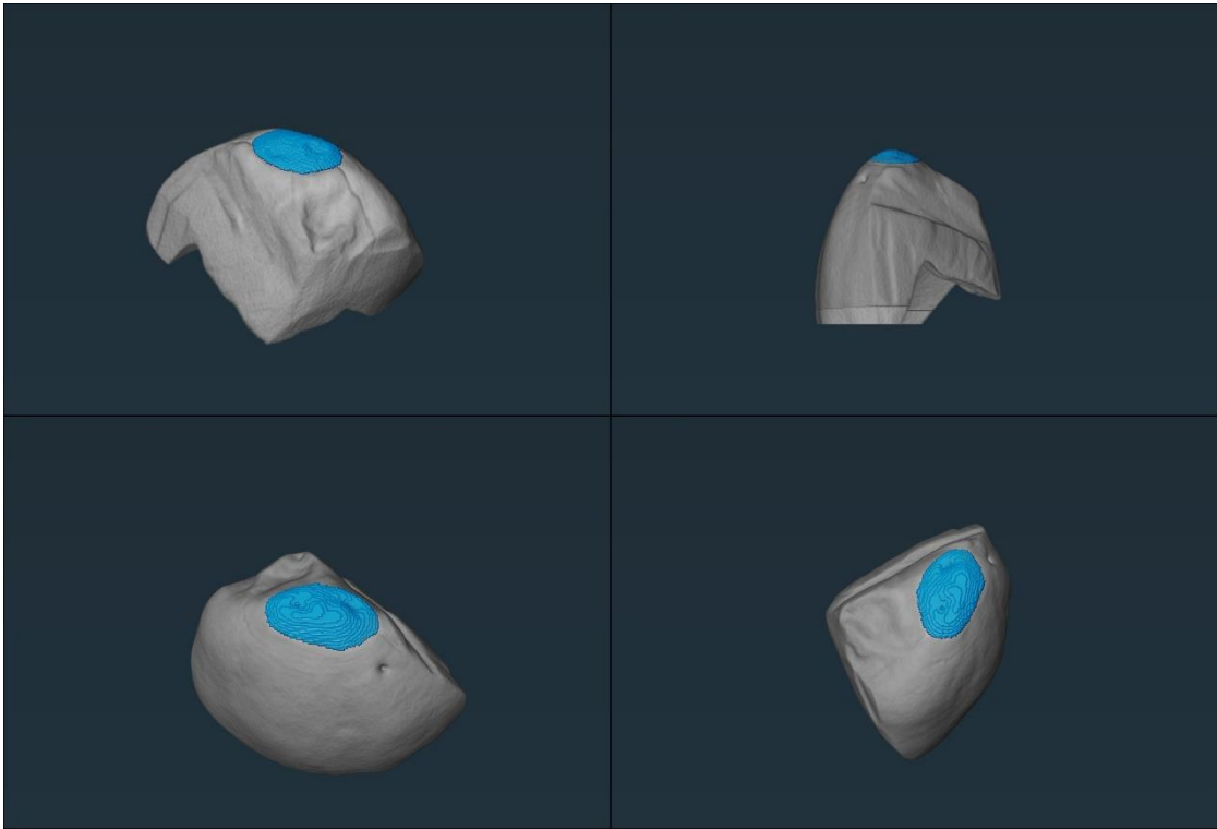
Figure 3: Abrasion (blue) on specimen 3
