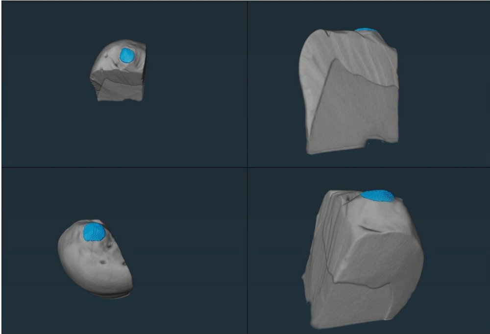
Figure 1: Abrasion (blue) on specimen 1
