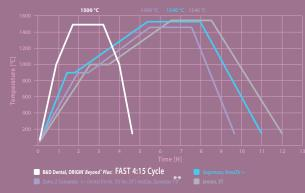
\*\* Up to 3 unit bridges. Larger restorations will require longer sintering cycles.
