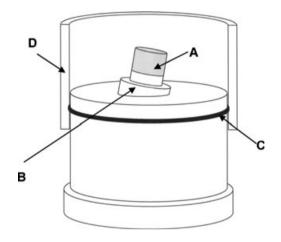
**Fig. 3.** Jig used for pre-loading and loading tests. A, Norm crown mounted in the jig; B, Brass foundation; C, Rubber gasket and D, Brass cylinder for water storage (shown cross-sectioned).
